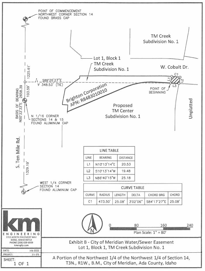
P:\Z1-172\CAD\SURVEY\EXHIBITS\Z20725 TM CREEK WATER-SEWER EASEMENT 21-172.DWG, TREY ZIMMERMAN, 7/26/2022, DWG TO PDF.PC3,
